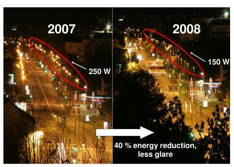
Two photos of Tržaška Road in Ljubljana: The left photo is from year 2007 with old luminaries using 250 W HPS bulbs. To the right is the situation in 2008 showing reconstructed road illumination using 150 W HPS bulbs with fully shielded luminaries, as stipulated by the Decree on the limitation of light pollution of the environment. Energy consumption has decreased by about 40% and emissions over the horizontal are 0%.
